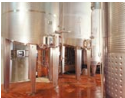
Self-emptying Conical Bottom
