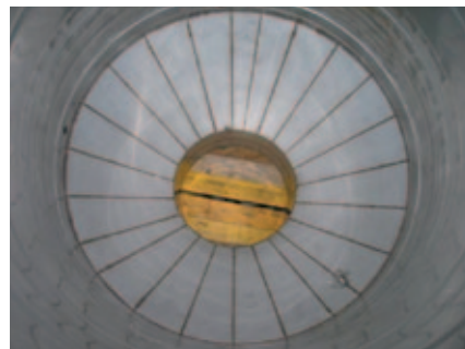
4) Internal welding of the segments to create the funnel-shaped diaphragm: the “funnel” diaphragm is reassembled following an accurate welding process performed by qualified personnel.
