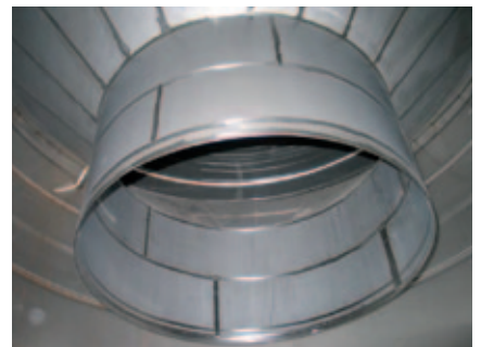
4) Internal welding of the segments to create the funnel-shaped diaphragm: the “funnel” diaphragm is reassembled following an accurate welding process performed by qualified personnel.
